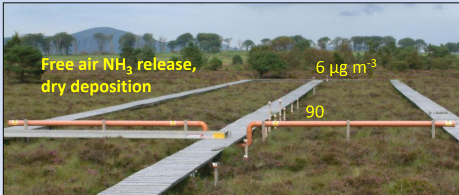
Whim Bog (UK) Free air fumigation with reduced and oxidized N deposition
